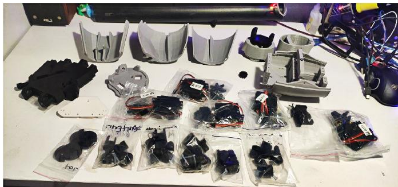
Figure 7 All Hardware Parts of the Gripper Prototype
