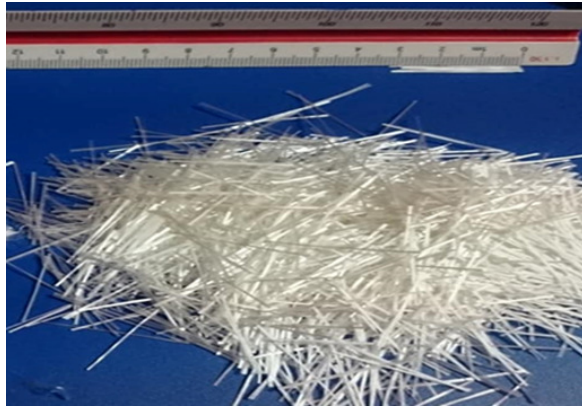
Fig. 1. AR glass fibers sample: 30mm length (A).
